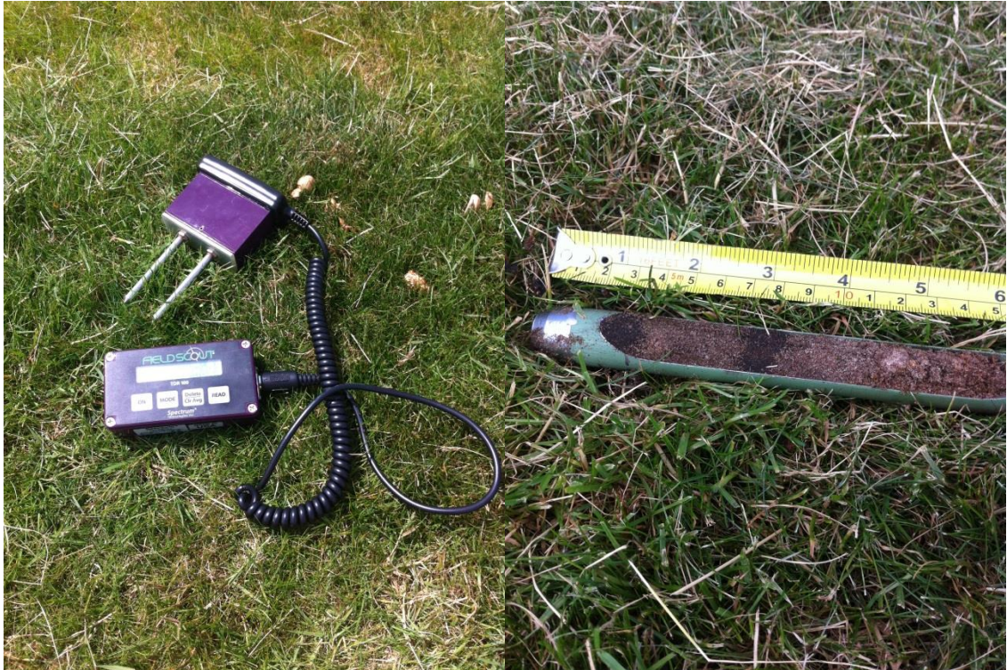
Figure 71: Fieldscout TDR 100 soil moisture meter on the active zone of a M. oroades fairy ring with the 7.5 cm length rods fitted
