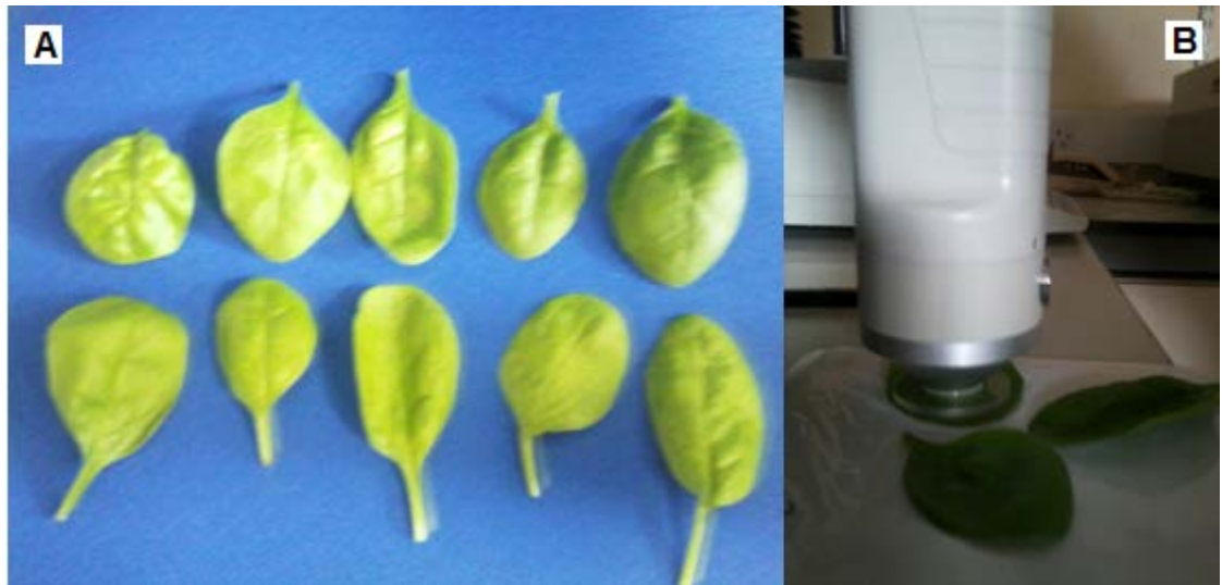
Plate 2.3 (A) Sample of spinach leaves showing uniformity of leaf colour. (B) Taking measurement of spinach leaf colour using Minolta.
