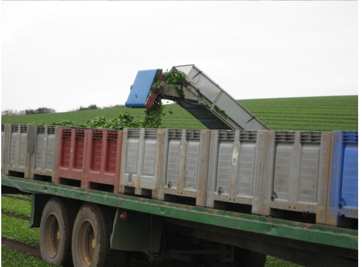
Plate 1.3 Process of mechanical harvesting of spinach leaves. (A) A machine with a front cutter bar runs on the top of the plant beds. (B) The leaves are lifted by conveyor belt into bins on trailers.
