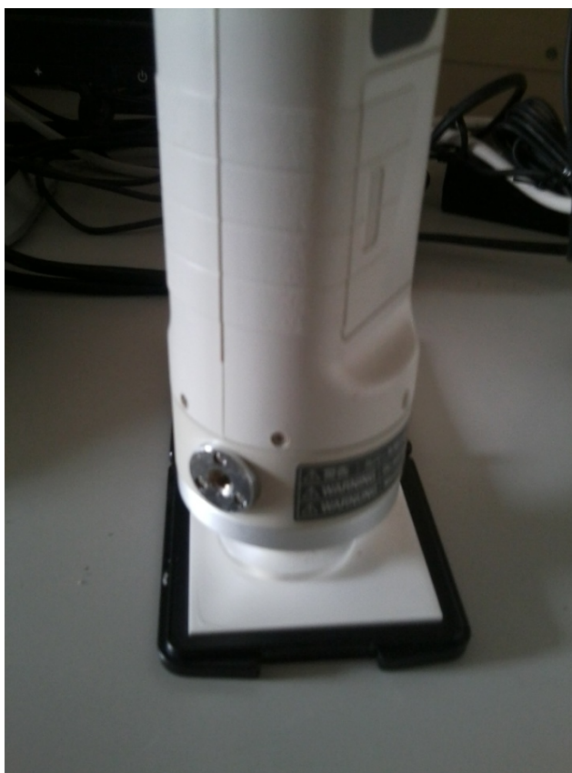
Plate 2.2 Minolta being calibrated using the manufacturer's standard white plate.
