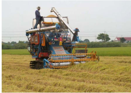
(b) A heavier tanker harvester on a firm plastic soil
