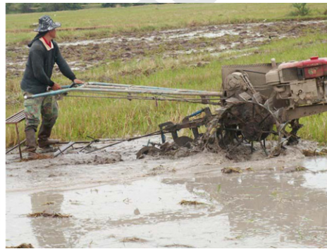
(a) Primary cultivation with a two disc plough –flooding started when cultivation started
