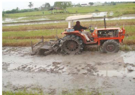
(d) Primary cultivation with a rotavator but little wheel sinkage
