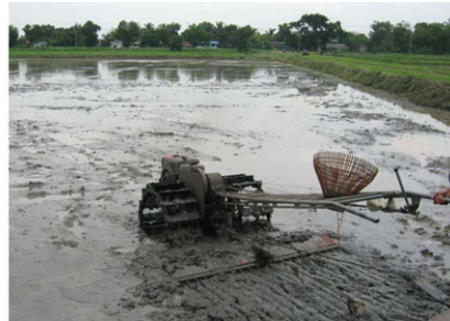
(b) Peg tooth harrow (left), puddling with a peg tooth harrow (right)
