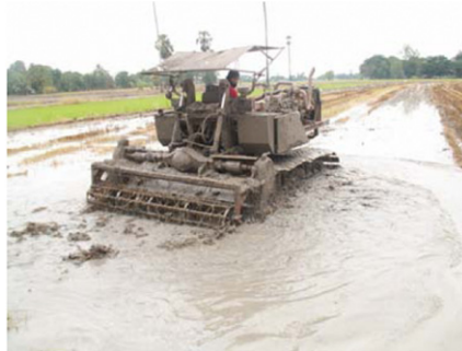
(f) A heavy tracked vehicle with a rotavator in soft soil paddy filling with water
