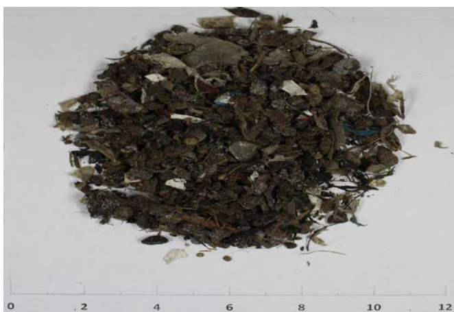
Fig. 4. The organic fraction of municipal solid waste prior to pyrolysis (Source: Fraunhofer UMISCHT, pers. Comm.)
