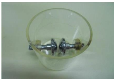
Figure 1: Test cell for breakdown voltage test of biodegradable oil sample.
