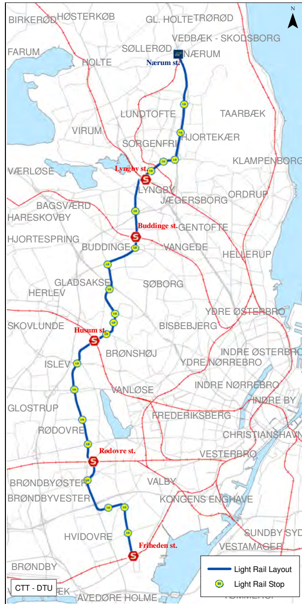
Figure 3 – Final alignment and locations of stops of the Ring 2½ light rail
