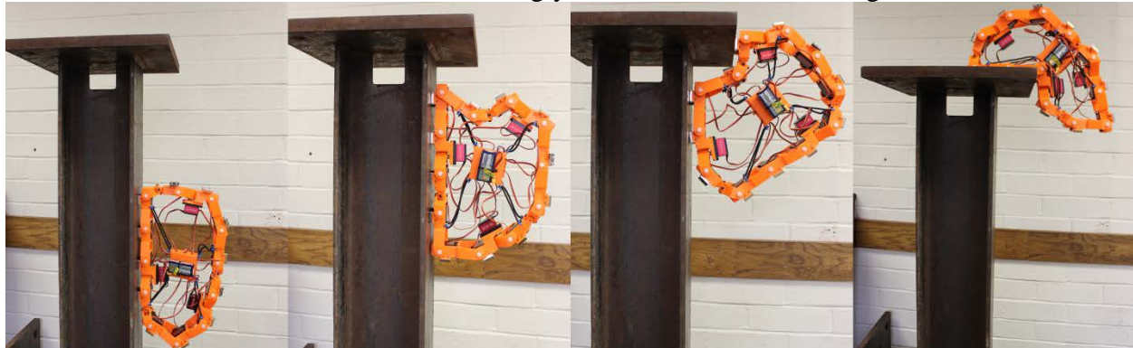
Fig 13. Climbing tests on steel structures. Video demonstration: https://ara.cse.unr.edu/?page_id=11
