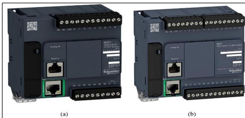
**Figura 46- 2:** (a) PLCs Schneider TM221CE16T y (b) TM221CE24T.
