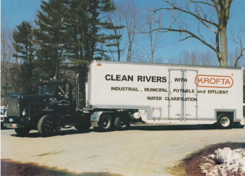
Figure 1. Krofta Engineering Corporation's DAF-filtration pilot trailer (Sandfloat Type SAF-BP-5; 5-inches diameter)
