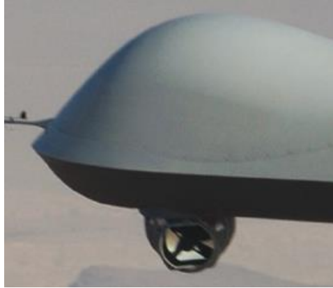
Figure 1. Gimbal on underside of unmanned aerial vehicle (UAV) 1
