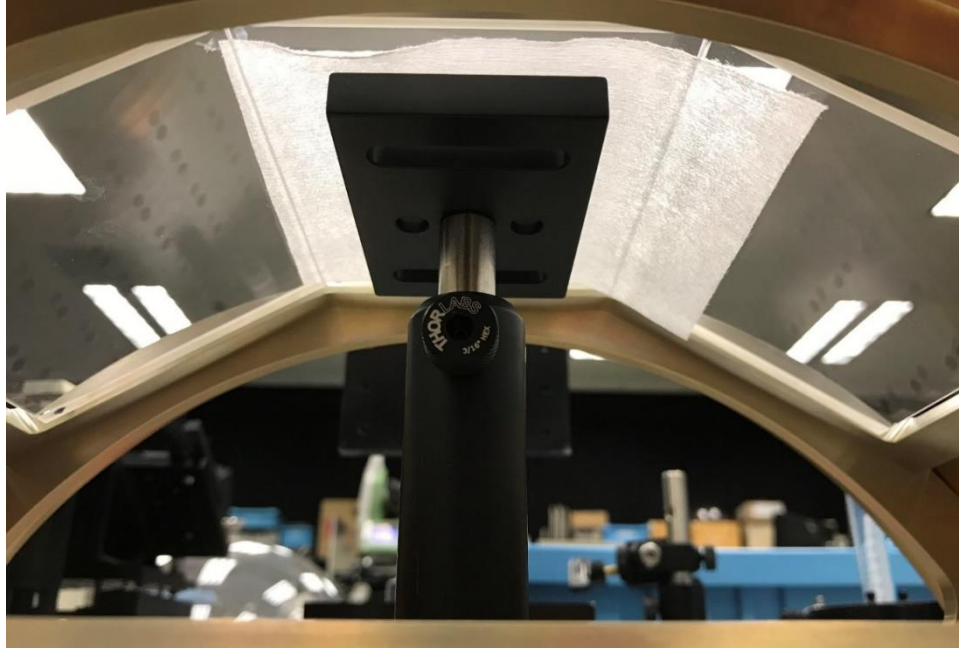
Figure 18. Window sub-assembly supported within frame from beneath
