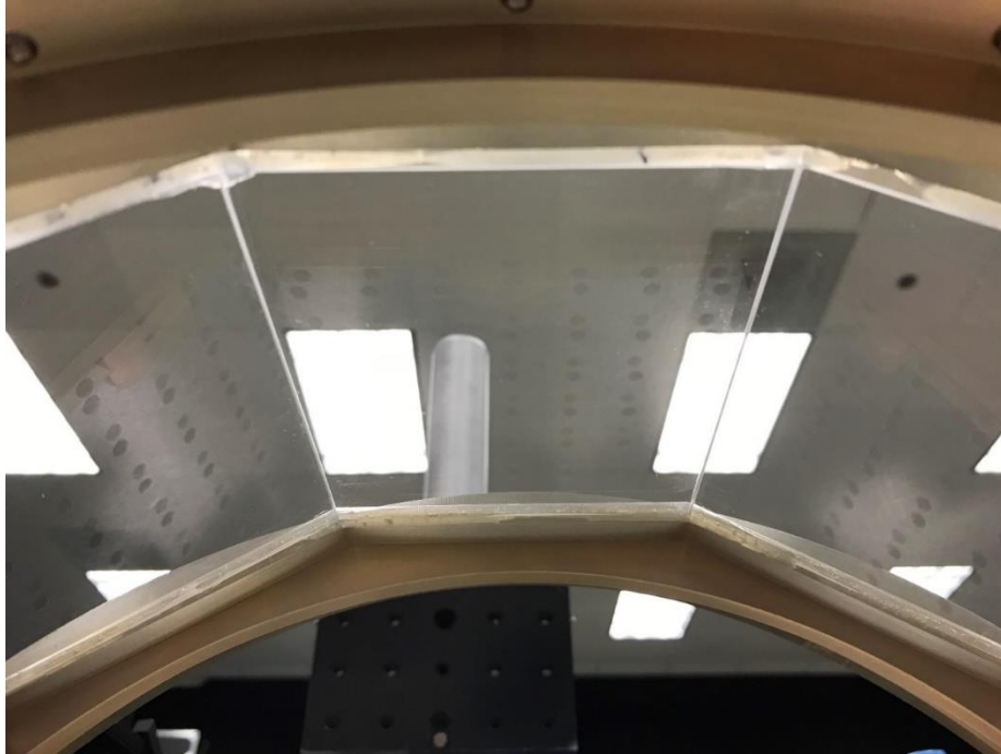
Figure 22. Near-conformal window assembly prototype, from inside
