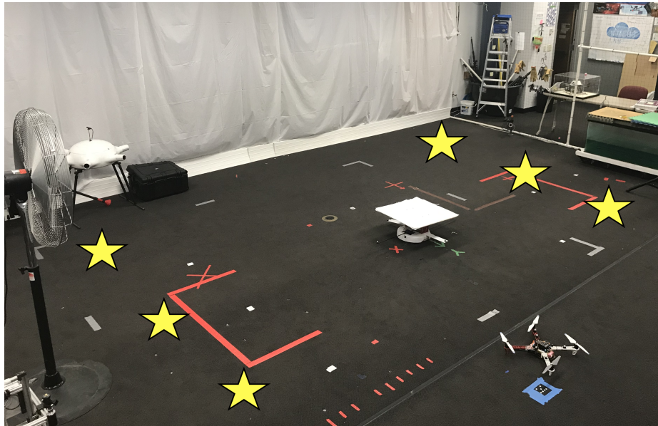
Figure 5.1: Experimental setup of the real-world experiments. The yellow stars mark the six initial positions that are initialized twice during an experiment. At the left of the image is the fan used to generate the disturbance; bottom-right shows the UAV used in the landings and, at the center, the Roomba robot with the moving platform.
