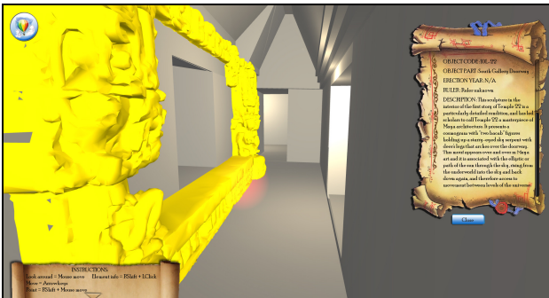
Figure 15: Example of a query on a single building at LoD2: information regarding the architectural element of the interior doorframe (as a whole) is shown.
