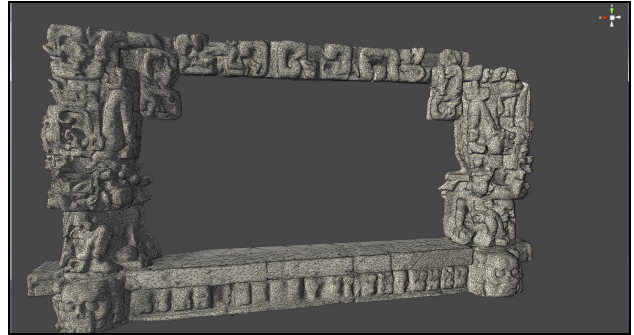
Figure 11: Detail view of the interior doorframe at LoD4: due to the large number of triangles used in the model, visualisation of LoD4 elements takes place separately.
