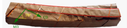
Figure 11. Transposed strand of the CTC and paper layer 1 in Ageing State IV and d = 5 mm.
