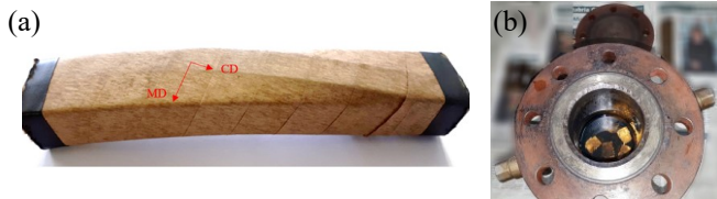
Figure 1. (a) CTC sample with the principal directions of the paper, MD and CD; (b) test pieces in the vessel filled with dielectric oil.
