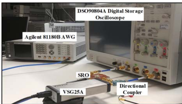
Fig. 15. Photograph of the measurement setup. The RF input signal is generated using the vector signal generator VSG25A, which provides an ASK modulated input signal with the power of P_{RF} = -10 dBm.
