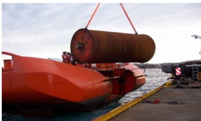
Figure 5: Installation of a Stern Roller. Source: Sotra Contracting AS.
