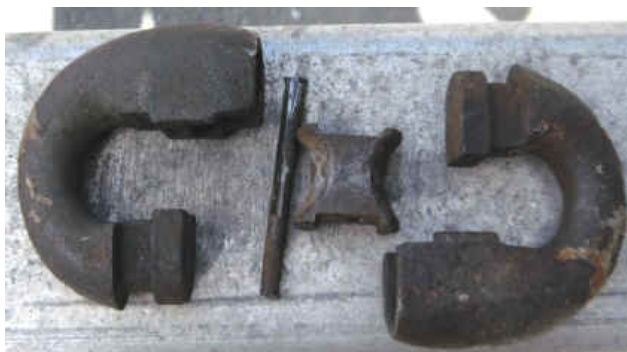
Figure 14: : Opened Kenter link. Source: Blue Ocean Tackle.
