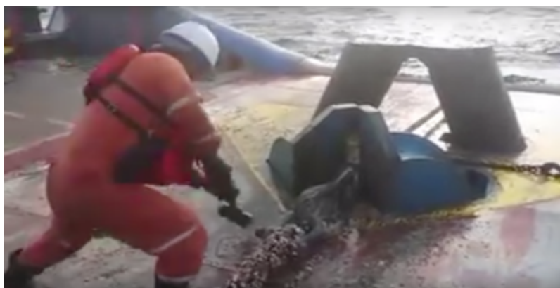
Figure 46: Deck crew member with a wrench disconnecting the thread in a shackle.
