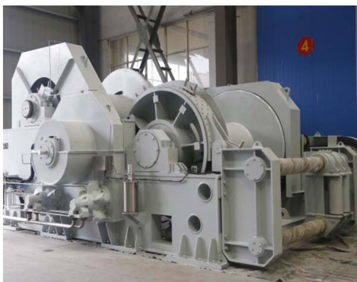
Figure 1: Main towing winch or Anchor Handling winch. Source: Wuxi Delin Marine Equipment.
