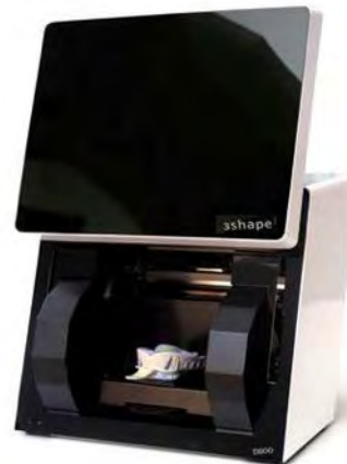
Figure 2. Laboratory scanner creates a 3-dimensional set of points by information of sectioned cast or impression.
