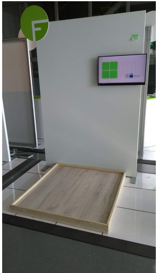
Figure 1: Prototype solution using off-the-shelf sensors under a standard laminate floor. Arduino Mega collects all the data and a program on a notebook running all our algorithms visualizes possible fall situations.
