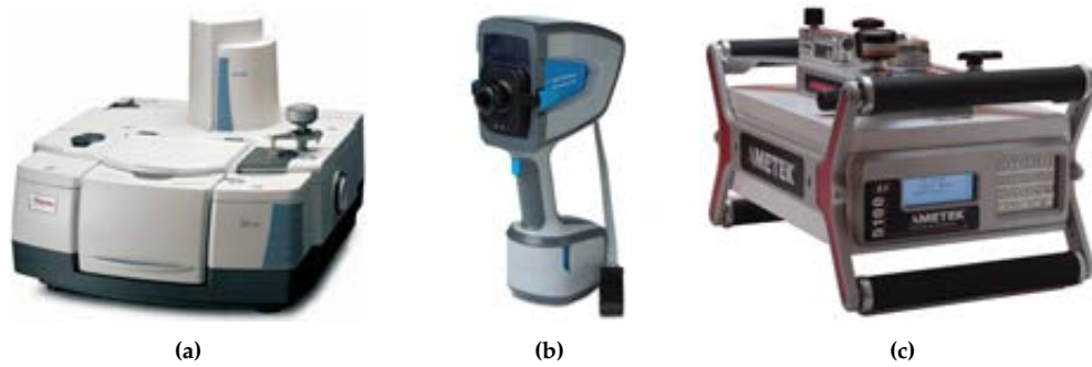
Figure 1.7: Examples of commercial spectroscopy systems. (a) Benchtop FTIR model, Thermo Scientific's Nicolet iS 50 FTIR [42]. (b) Handheld FTIR model, Agilent's 4300 Handheld FTIR [43]. (c) Portable TDLAS gas analyzer, AMETEK's 5100P TDLAS [44]. The three images have different scales.
