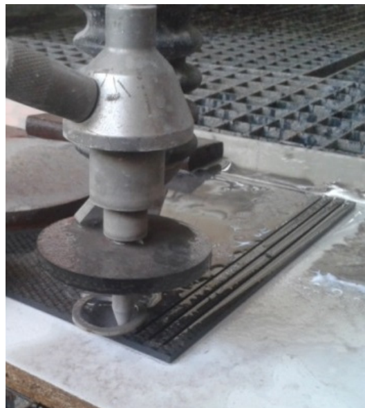
Figure 1. Mecanumeric MECAJET performing carbon fiber reinforced composite material with a polymeric matrix (CFRP) cutting.
