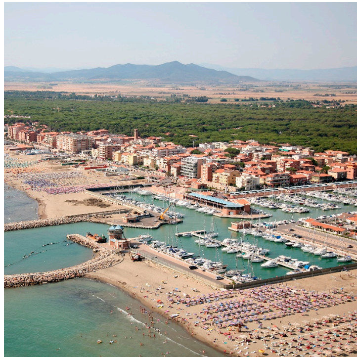
Figure 8. The boathouse at Marina di Grosseto, whose entrance is protected by two jetties. The updrift one intercepts the long shore sediment transport, creating an extensive beach.
