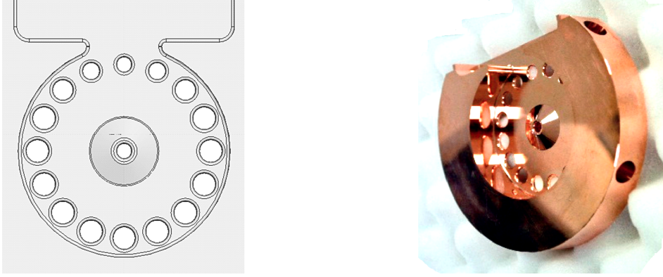
Figure 2.2: Input coupler design (left) and single mechanical cell (right) of the S-band BTW HT.
