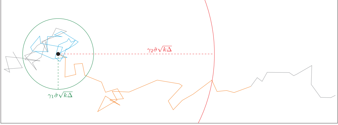
Fig. 1. Illustration of the detection step of the candidate change-points with k=30 and n=90 . The 2D trajectory is Brownian for i \in \{0, \dots, 60\} , after the process is a Brownian motion with drift. The change-point \tau_1 = 60 is represented by the black dot. The blue (respectively, orange) part corresponds to the subtrajectory \mathbb{X}_{\tau_1}^- , respectively, \mathbb{X}_{\tau_1}^+ . Comparing the test statistics (7) to (\gamma_1, \gamma_2) is equivalent to determine which area, delimited by the red and green circles centred on X_{\tau_1} , the particle reaches. The blue subtrajectory stays inside the inner circle: it is classified as subdiffusive. The orange subtrajectory goes outside the outer circle: it is classified as superdiffusive. This point is detected as a potential change-point
