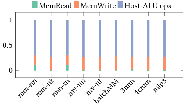
Figure 7. Instruction breakdown for the baseline without offloading.
