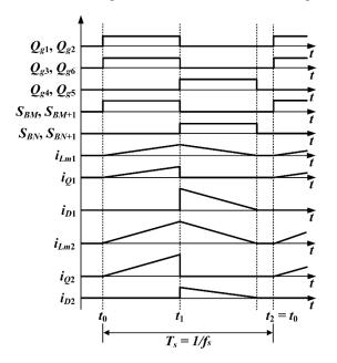
**Figure 4.** Operation waveforms of proposed active balancing circuit for pack-to-odd cell and even cell-to-pack operations.
