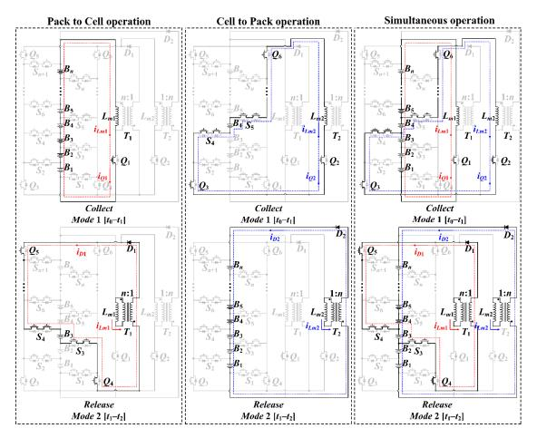
Figure 3. Operation modes for pack-to-odd cell and even cell-to-pack operations.
