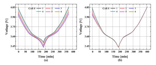
**Figure 12.** Voltage versus time under the one cyclic discharging/charging period: (**a**) without charge equalization, (**b**) with charge equalization.
