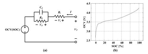
**Figure 5.** (a) Equivalent circuit of the Li-ion battery cell and (b) OCV (state of charge (SOC)): OCV versus SOC characteristic of the experimental Li-ion cell.
