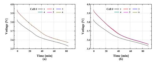
**Figure 11.** Voltage versus discharging time for the battery pack: (**a**) cell-to-pack balancing in discharging operation and (**b**) pack-to-cell balancing in discharging operation.
