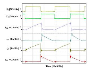
Figure 8. Operational waveforms of the proposed balancing circuit.
