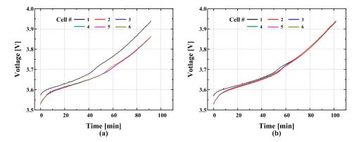
**Figure 10.** Voltage versus charging time for the battery pack: (**a**) pack-to-cell balancing in charging operation and (**b**) cell-to-pack balancing in charging operation.
