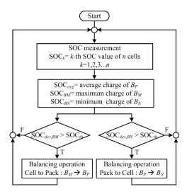
Figure 6. Balancing algorithm for the proposed balancing circuit.
