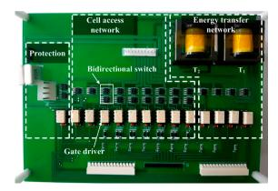
Figure 7. Prototype of the proposed balancing circuit for equalization of six cells.
