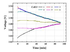
**Figure 9.** Voltage versus balancing time for the proposed charge equalization; six cells were connected in a static condition.
