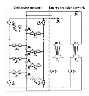
Figure 2. Circuit structure of the proposed active balancing circuit using double energy carriers.
