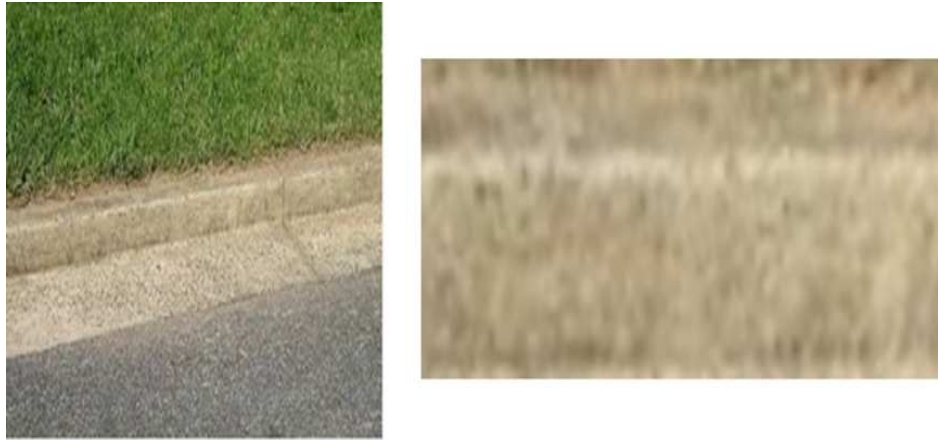
Fig. 4.19. Pattern 3. Real curb (Left), Example Pattern of 6 inches Wide, 6 inches Tall and 24 inches Long (Right)
