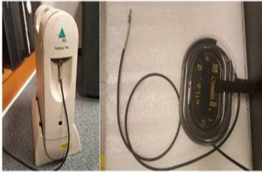
Fig. 3.13. ASD FieldSpec Pro Spectrometer (Left), Optical Fiber Probe (Middle), and 1° Field-of-View Reducer Accessory (Right)
