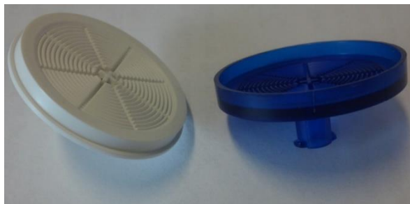
Figure 34: Cyrolite® membrane housing for ILC measurements.
