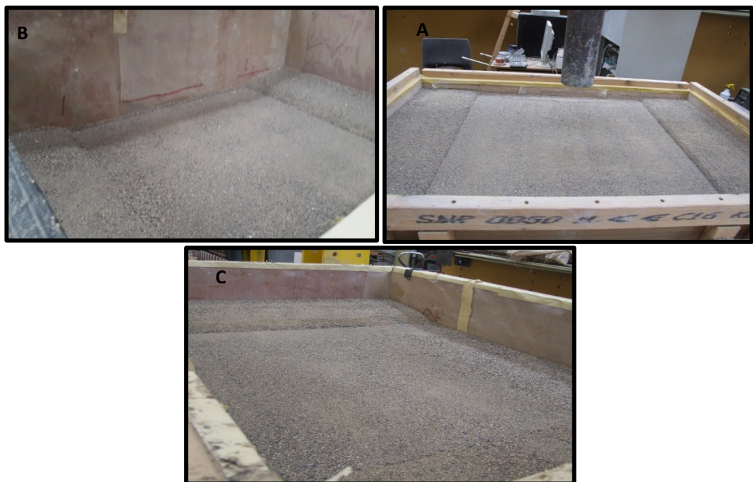
Figure 6.33. Soil surface settlement after removing the applied loads of three layers reinforced embankment (A) 200 mm (B) 400 mm and (C) 600 mm.
