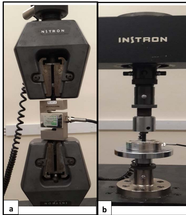
Figure 3.15. Calibration of load cells (a) tension load cell (b) compression load cell.
