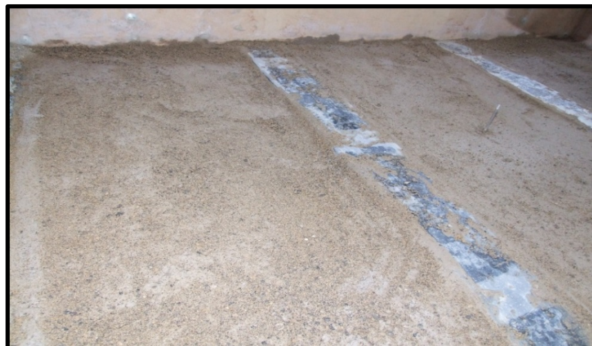
Figure 6.35. Deformations at the soft soil surface after completion of test of 200 mm unreinforced embankment.
