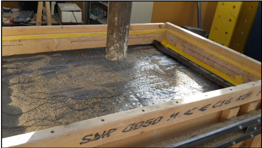
Figure 3.29. Reinforcement layer before filling the embankment soil into the box test.
