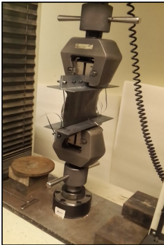
Figure 3.27. A wide-width tensile test for the used geotextile reinforcement material.
