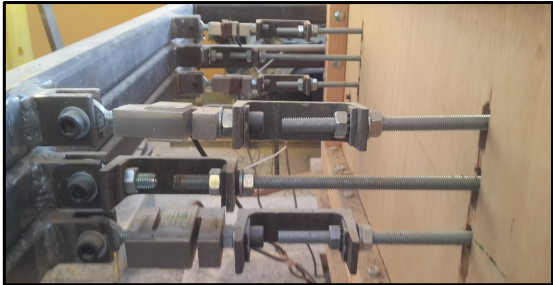
Figure 3.14. System of measuring tension in reinforcement layers.
