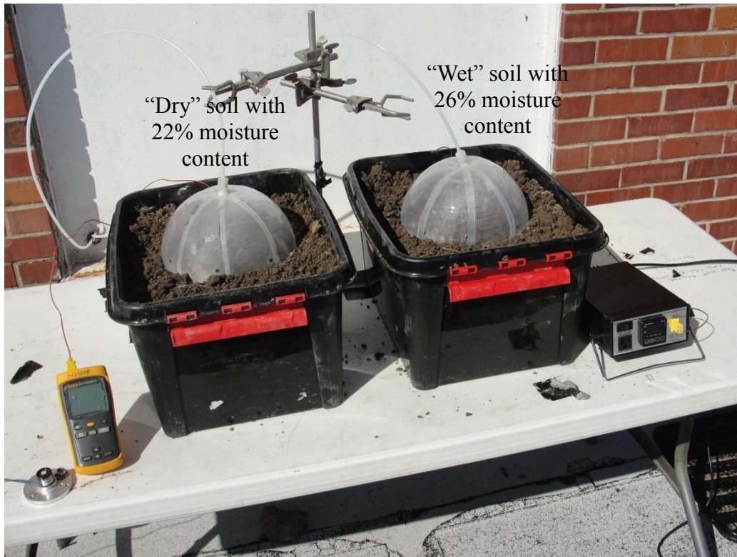
Figure 28. Experimental setup comparing mercury fluxes over dry and wet soils Emission fluxes over wet and dry soils was evaluated. The relative concentrations (wet/dry) of mercury over the two soils is shown in Figure 29. Mercury fluxes over the wet soil initially decreased (for about 2 hours) but then returned to about the same level as the drier soil during the night. The decrease is agreement with other studies (Bahlmann et al. 2006; Kockman et al. 2010) and may stem from water impeding mercury desorption from soil (lowering diffusivity). Bahlmann et al (2006) also proposed that decreased Hg flux was due to a combination of soil moisture tension and soil moisture. In their study, after wetting the soil they allowed the water to percolate through the soil column. The soil moisture tension in the surface layer became weaker, resulting in less Hg enriched soil air being displaced and less Hg being desorbed from the soil surface.
