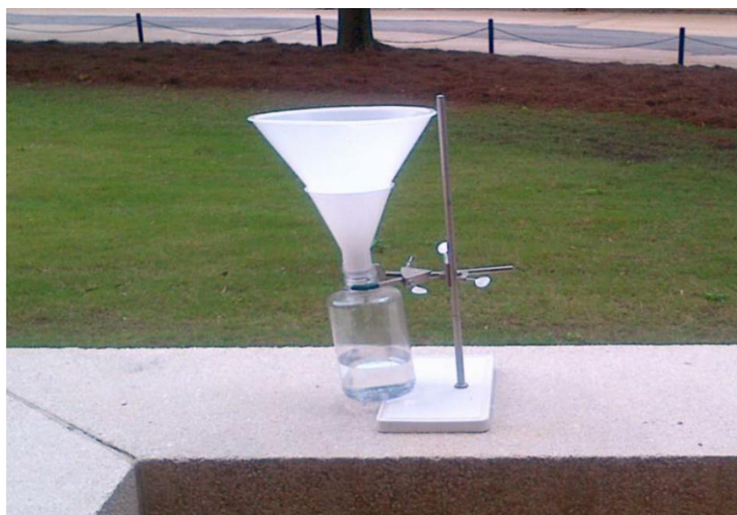
Figure 30. Rainwater collection apparatus outside of Coulter Hall on the University of Mississippi campus
