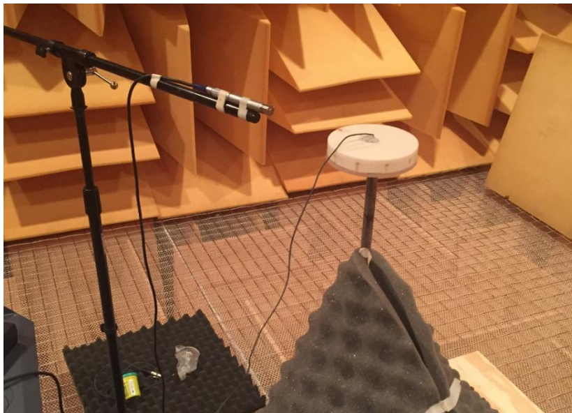
Figure 2.7. Measurement of the sound pressure field in the presence of the structure
