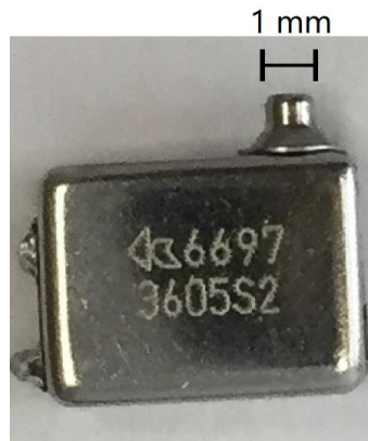
Figure 2.4. Model CI-26697-000 Knowles balanced armature speaker
