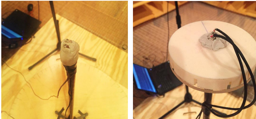
Figure 4.12. Measurement of the sound pressure field in the absence of the structure (left), and presence of the structure (right)
