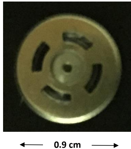
Figure 4.2. Up-today, DS98001-000 dynamic speaker with 0.9 cm diameter
