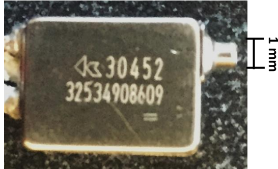
Figure 4.11. Model CI-30452-000 Knowles balanced armature speaker
