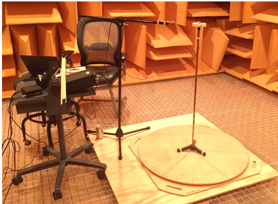
Figure 2.3. Experimental setup at the anechoic chamber at the National Center for Physical Acoustics (NCPA), University of Mississippi
