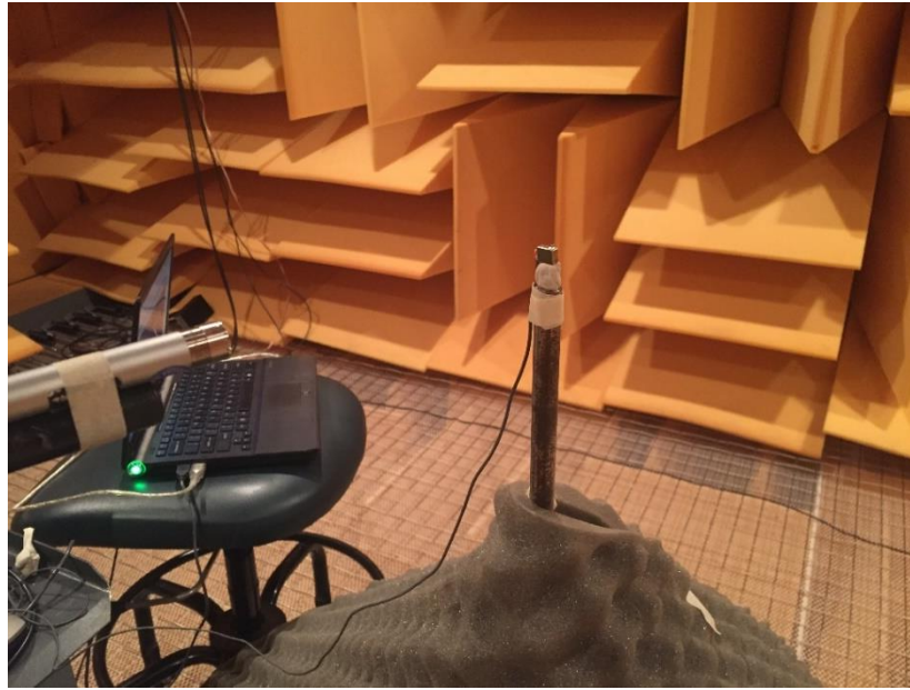
Figure 2.6. Measurement of the sound pressure field in the absence of the structure
