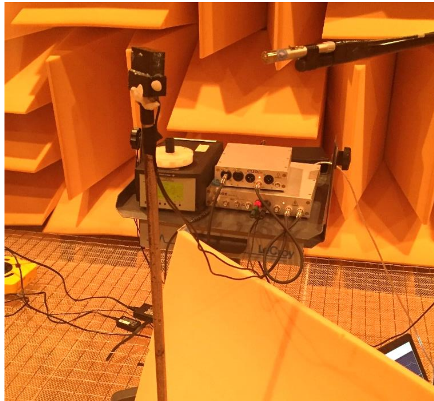
Figure 4.5. Measurement setup to for sound pressure field of the dipole with absence of the structure
