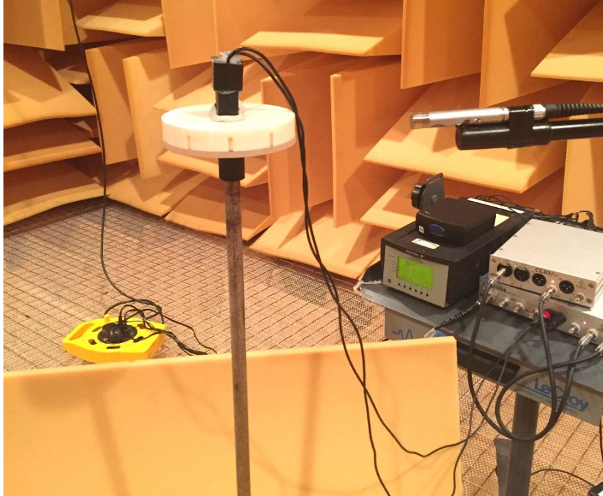
Figure 4.6. Measurement of sound pressure field of the dipole in the presence of the structure
