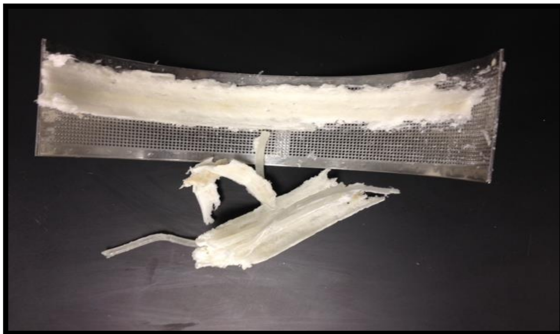
Figure 3-7: Failed milling of Klucel™ (ELF, EF, and LF) extrudates with PG injection.
