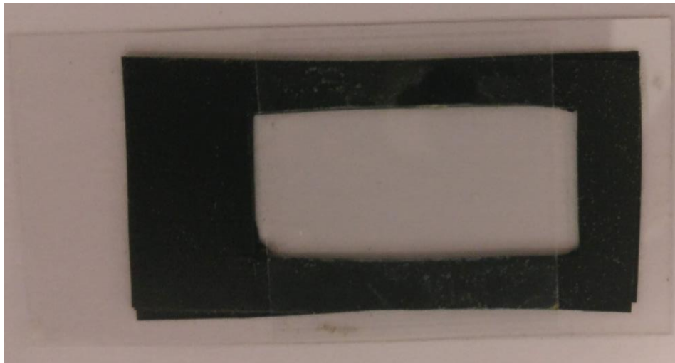
Figure 24: Elevation created using electrical tape on a coverslip for mounting anaesthetized zebrafish larvae for imaging under fluorescence microscope. The anaesthetized larvae were stable in this setting for 4-5 hours
