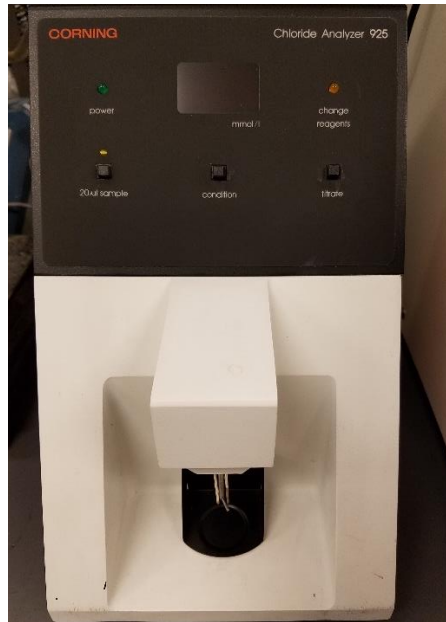
Figure 7: Chloride Analyzer (CIBA Corning 925 NSN 6630-01-137-8460)
