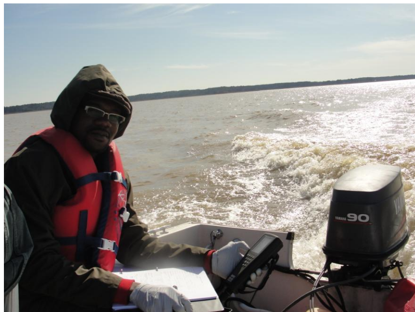
Figure 49 Collecting water quality measurements using the YSI multi-meter while traversing between sampling points on Enid Lake (stainless steel bucket with water not shown). Note turbid water and clear skies for best satellite imagery.
