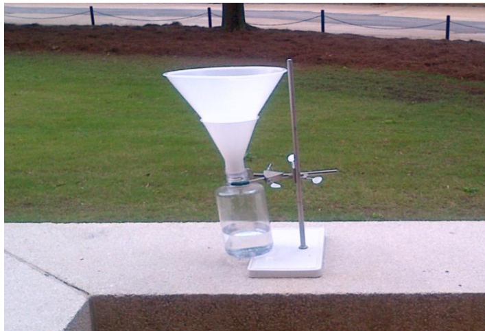
Figure 20 Rainwater collection apparatus (acid-washed LDPE funnels and 2 L polycarbonate bottle) outside Coulter Hall on the University of Mississippi campus.
