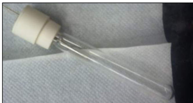
Figure 48. Picture of a 17 mL vial which has been equipped with a 24/40 stopper as septum, long steel needle as inlet needle, and short steel needle as outlet needle.
