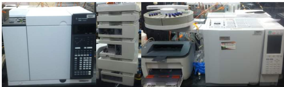
Figure 51. Left: Picture of the GC used for headspace analysis. Middle: Picture of the HPLC used for solution analysis. Right: Picture of the GC used for solution analysis.
