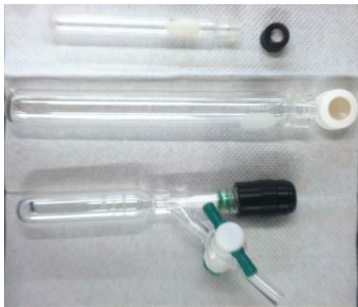
Figure 47. Top: 17 mL screw cap vial, Middle: 40 mL screw cap vial, and Bottom: heavy-walled schlenk flasks for use in photochemical CO 2 reduction.
