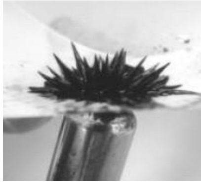
Figure 1.9 Ferrofluid under effect of magnetic field [42]
