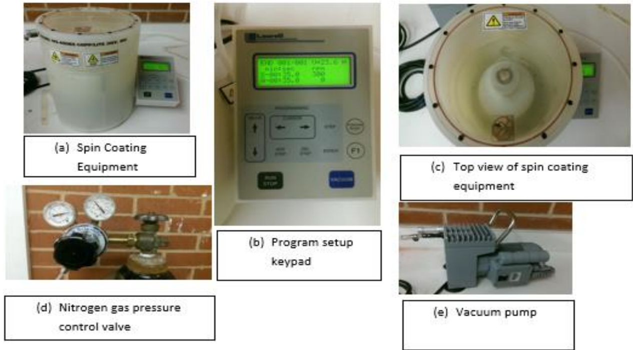
Figure 2.4 Actual setup of spin coating
