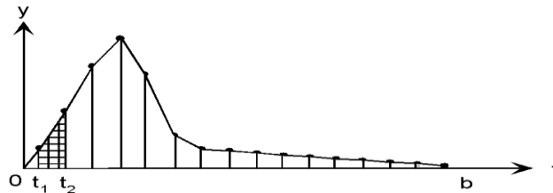
Figure 0.1 sample curve for calculation of area under the curve
