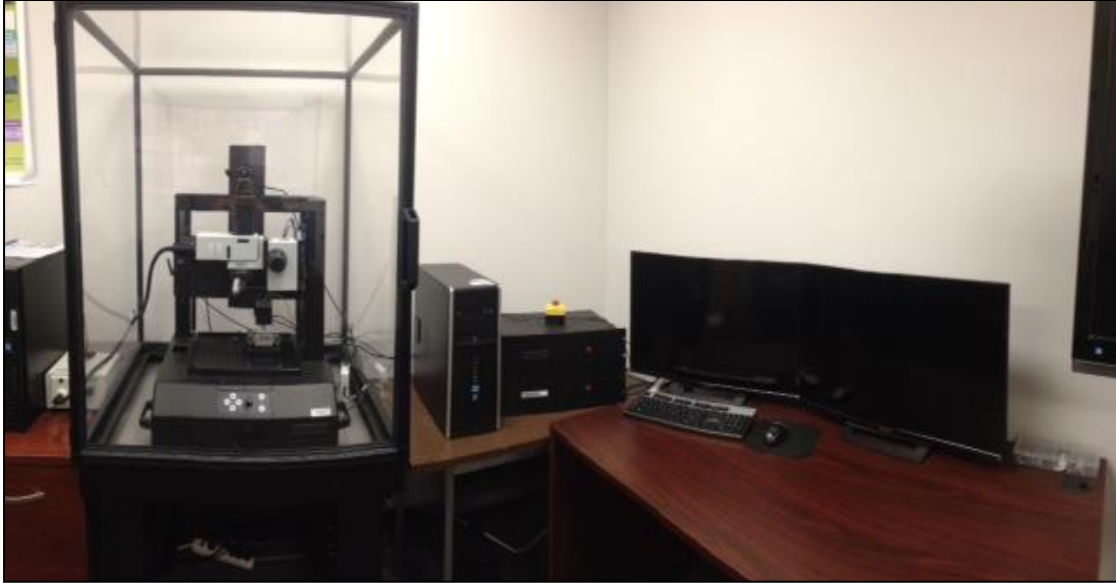
Figure 10: Nanovea M1 Hardness Tester with microscope, full set-up. Equipment is located within an isolation cabinet for the reduction of background noise. The cabinet is attached to the frame of an anti-vibration (air stayed) table which dampens any vibrations present within the interior or exterior of the cabinet itself.
