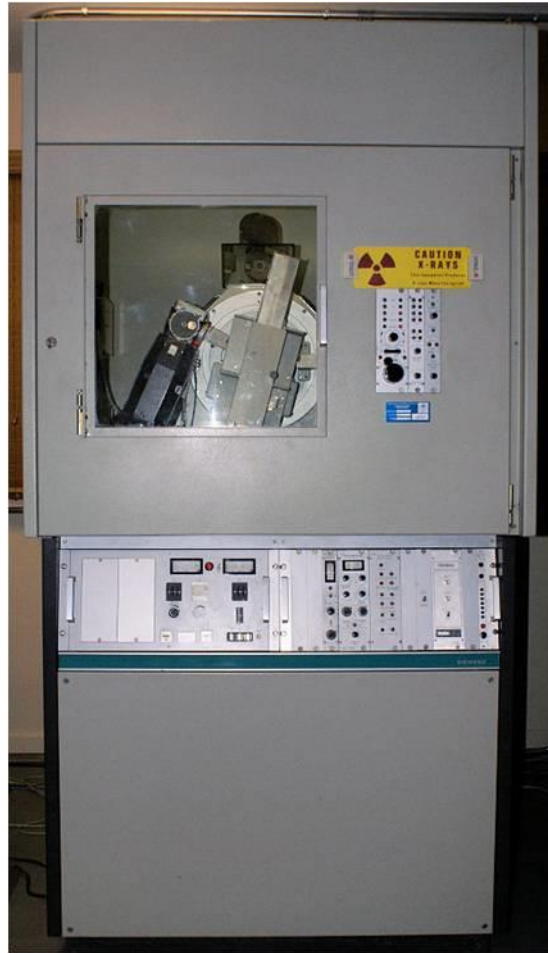
Figure 21: Siemens D500 automated powder X-ray diffractometer as used by K-T GeoServices (courtesy James Talbot, K-T GeoServices Inc.) (Talbot, 2012).
