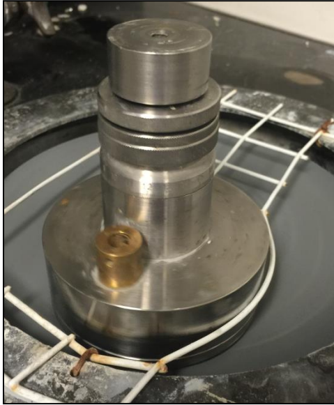
Figure 9: Polishing jig used to mechanically polish the specimen.
