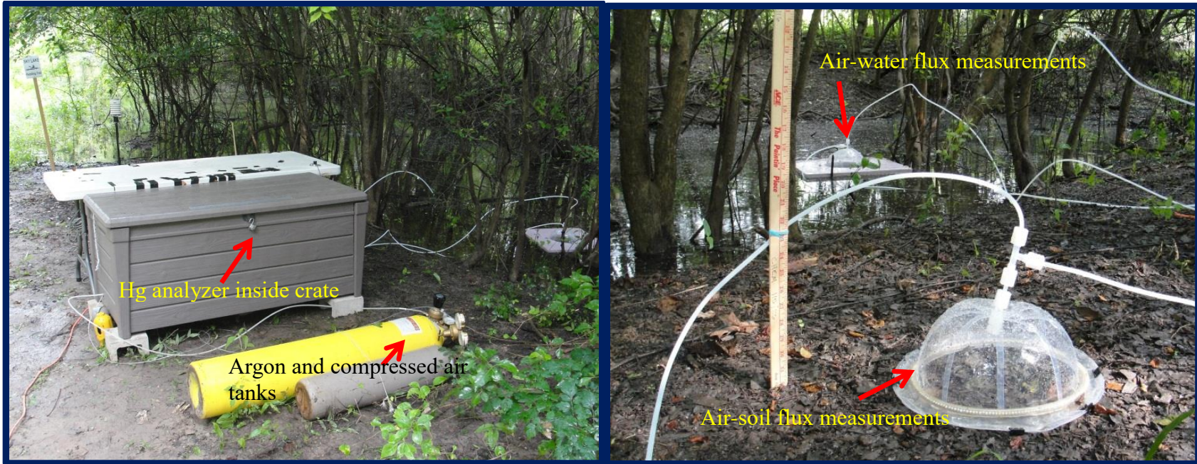
Figure 3. Experimental setup for measuring Hg flux over wetlands at Sky Lake. Dynamic flux chambers over water and soil can be seen on right.
