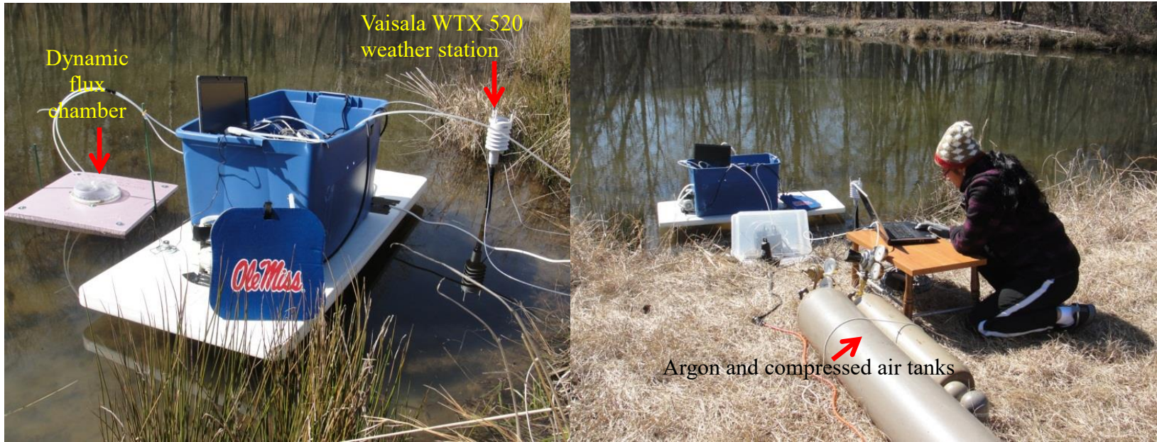
Figure 4. Experimental setup for measuring mercury flux over wetlands at the UM Field Station.
