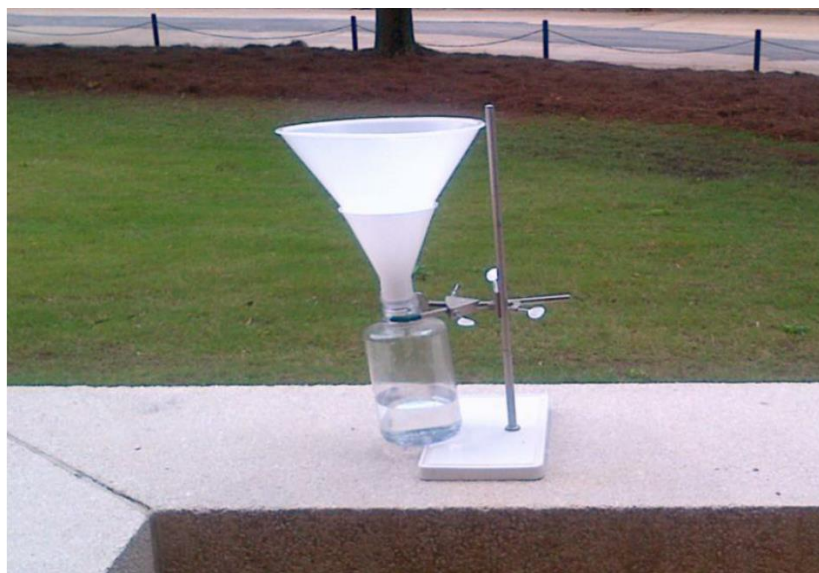
Figure 29. Rainwater collection apparatus outside of Coulter Hall on the University of Mississippi campus.
