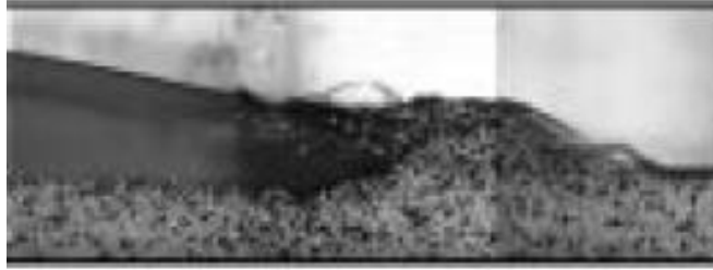
Fig. 5.11 Wave front with high sediment load at the initial stage of gate removal t=0.25 s (picture from Fraccarollo and Capart, 2002)
