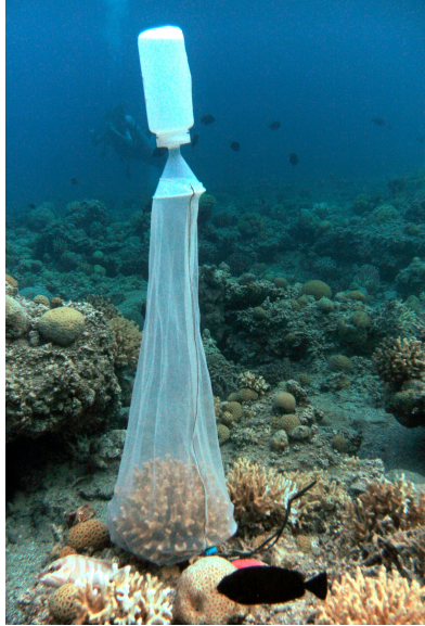
Figure 2. Planula collection net. Net is placed over a shallow water adult Stylophora pistillata colony.
