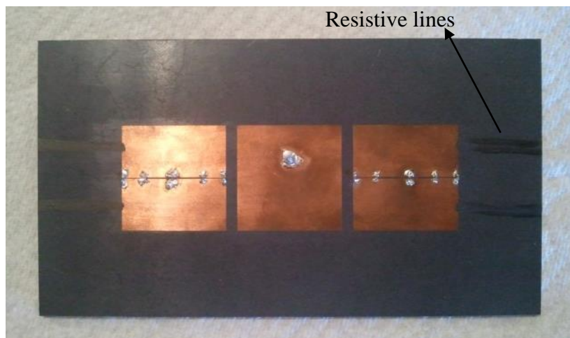
Figure 5-7. A photo for the proposed antenna fabricated prototype.
