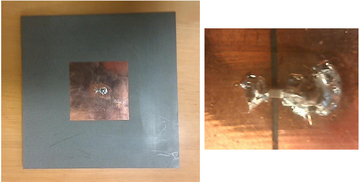
Figure 2-5. A photograph of the proposed patch antenna with a capacitor loaded-slot for dual-band operation.
