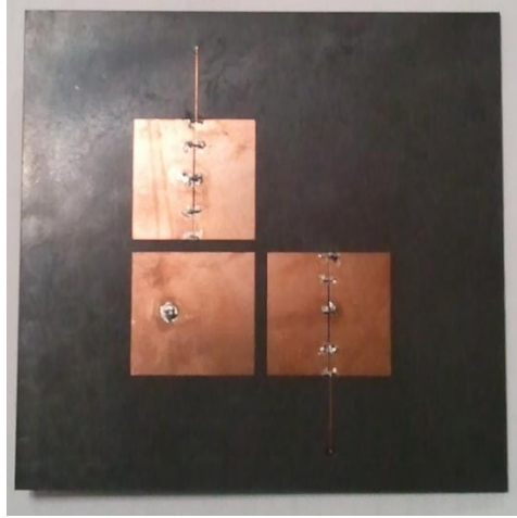
Figure 4-4. A photo for the proposed fabricated antenna prototype.
