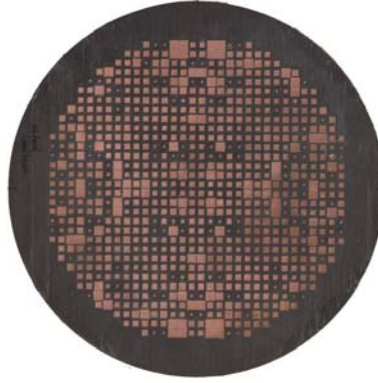
Fig. 5-15 Fabricated quad-beam reflectarray antenna.
