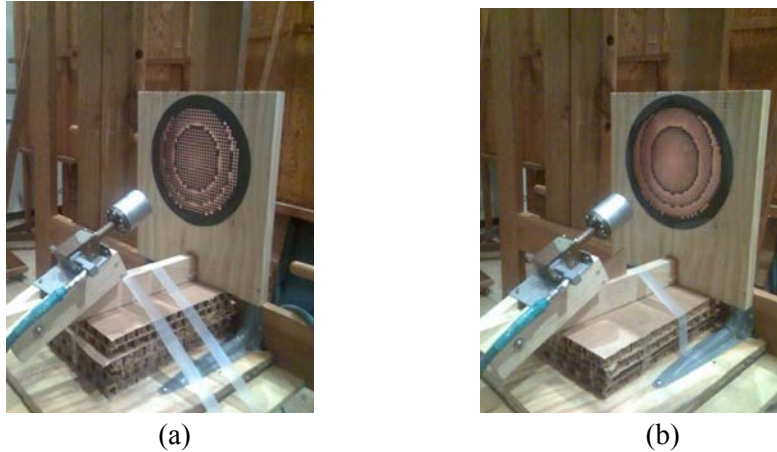
Fig. 3-5 Photographs of the fabricated arrays: (a) \lambda/2 array with 848 square patches, (b) \lambda/3 array with 1941 square patches.
