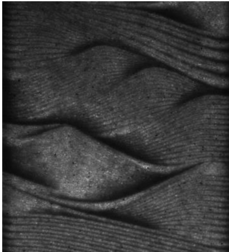
Figure 23. Sloping in layers occurs when the feeder tube does not move across the entire width of the chamber.
