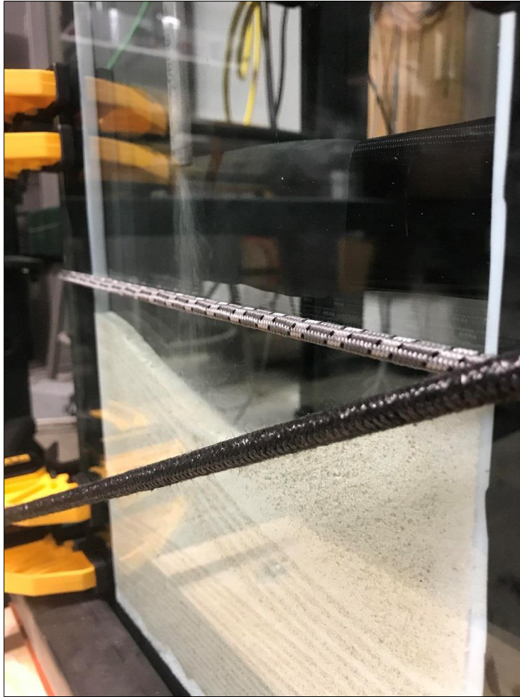
Figure 20. While filling the chamber sand is delivered at a constant flowrate and the feeder-tube is maintained at a constant drop height.
