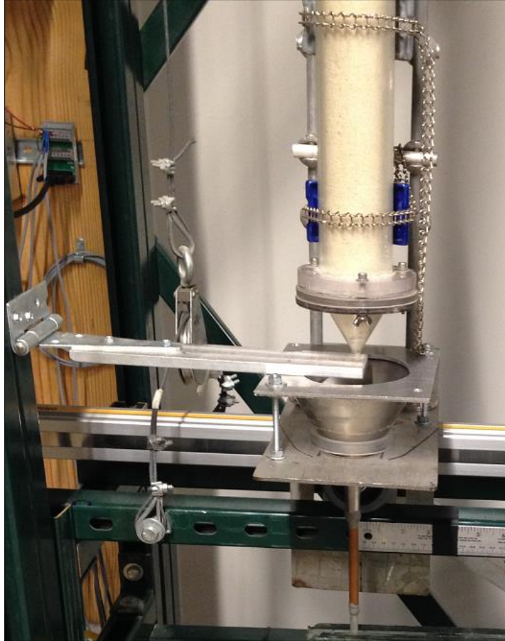
Figure 18. Randomized sand is held by a hopper that is housed on the sandfiller carriage, sand flow is impeded by a swinging gate.
