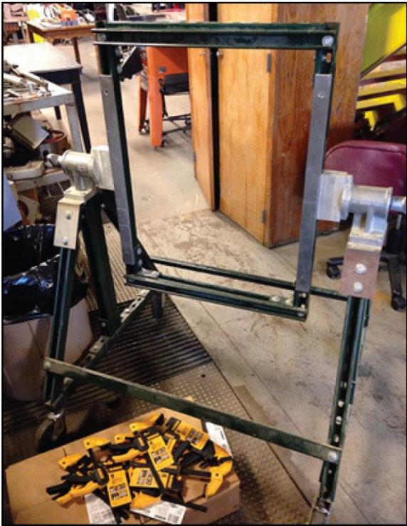
Figure 11. Rotating-visualization stage created from Unistrut metal framing systems with four casters to move the mount freely around the lab space. The diagram of the rotating-visualization stage with chamber and light panel attached. The arrows indicate portholes on the chamber and the flow direction of fluids.
