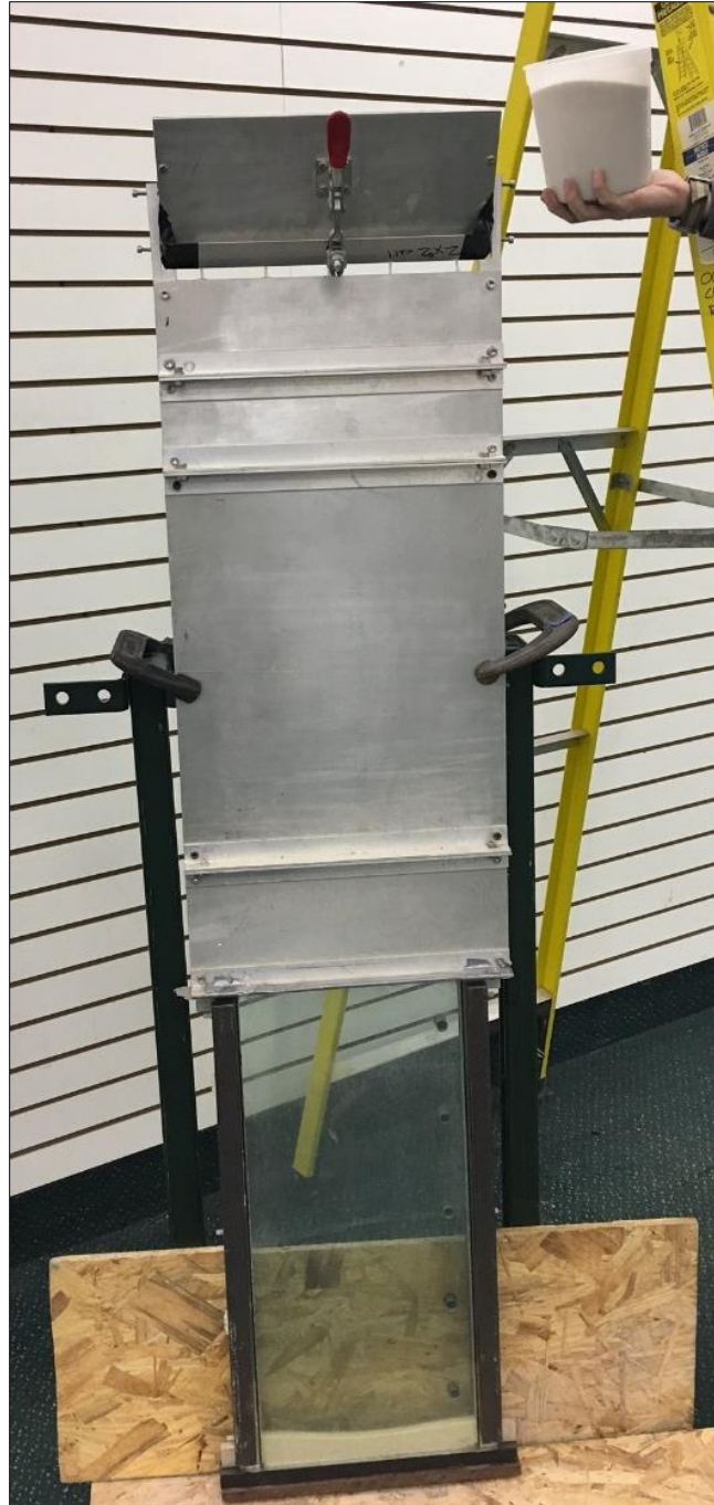
Figure 16. Creating homogeneous chambers by dumping sand directly through a rectangular randomizer with V-shaped trough.
