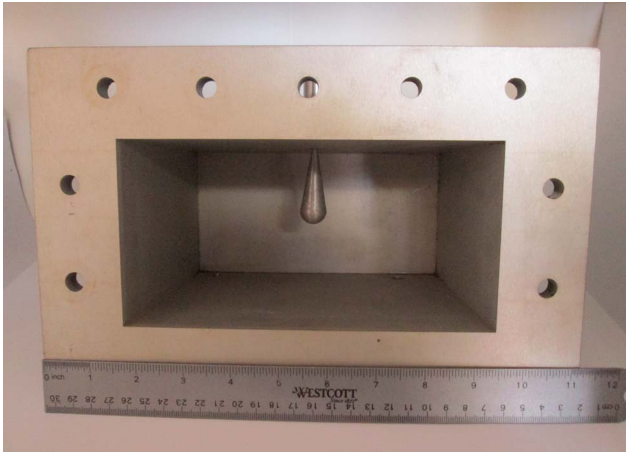
Fig. 4-28 WR770 waveguide adapter used to measure surface reflection.
