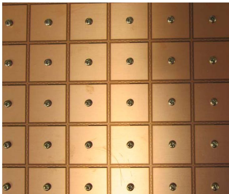
Fig. 4-26 Fabricated dual band EBG on 250mil Rogers Corp. TMM10 material.
