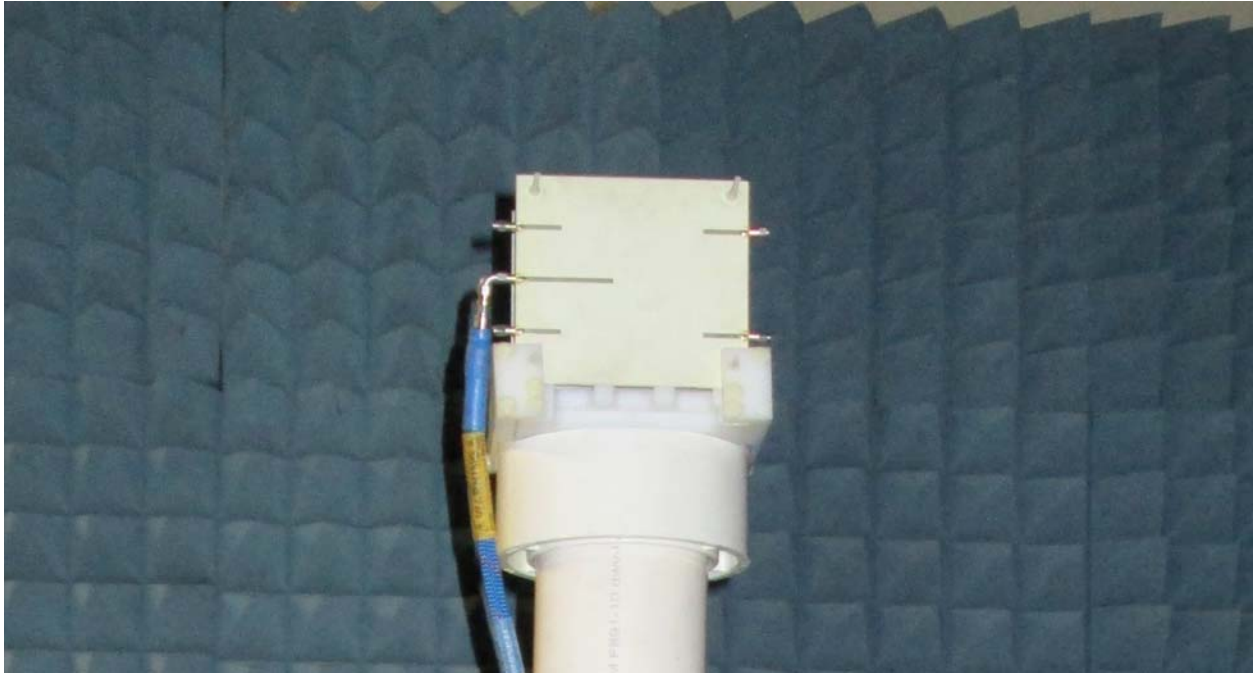
Fig. 3-9 Measurement setup for the 1 GHz linear horizontally polarized antenna in cylindrical near field scanner.
