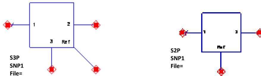
Figure 3.10 (a) discrete components for the 1:8 power divider in EM analysis
