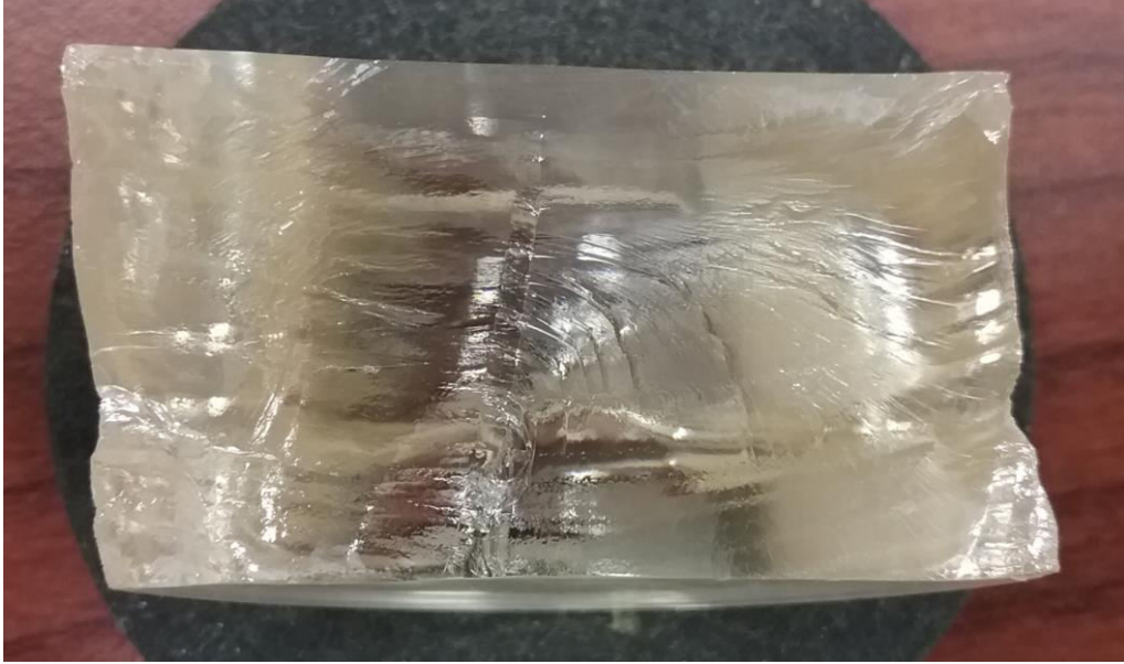
Figure 2-5. Macroscopic structure of domains on the cleaved diametric plane of LNO-U bulk crystal.
