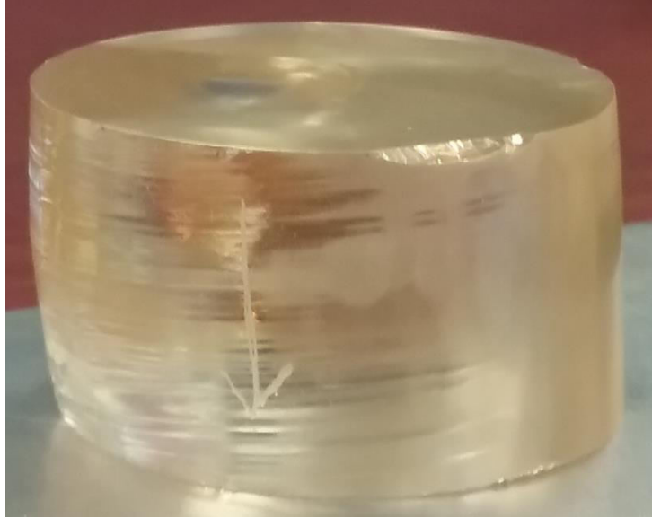
Figure 2-4. Macroscopic swirl defects on the outer face of LNO-P crystal. Polishing is performed towards the right to flatten out the grooves. The arrow shows the direction of the +z-axis.
