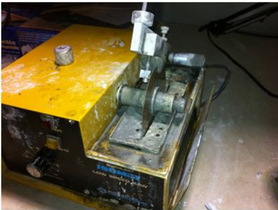
Figure 4.8. Cubes Are Cut in The Range of (1cm*1cm*1.5cm) Using a Diamond Saw , Polished for RUS, EIS, and Compressive Strength Testing
