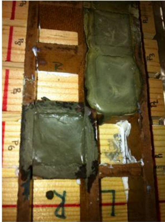
Figure 4.7. Cement Paste Casted in Cubical Molds (1.5"*1.5*1.5)
