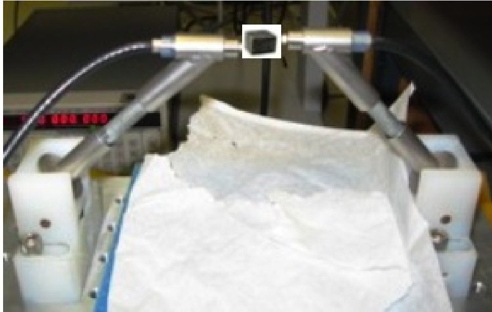
Figure 4.65. Room Temperature RUS Experiment Setup
