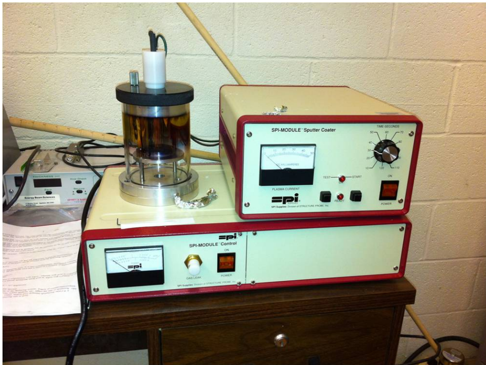
Figure 4.55. Sputter Coating Setup for SEM sample Preparation
