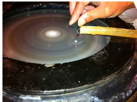
Figure 4.8. Cubes Are Cut in The Range of (1cm*1cm*1.5cm) Using a Diamond Saw , Polished for RUS, EIS, and Compressive Strength Testing
