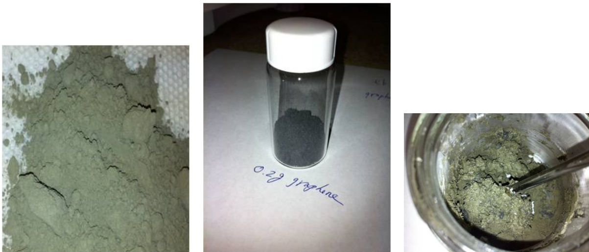
Figure 4.6. Preparing Cementitious Nanocomposite Paste (a)Portland Cement Type I/II Powder, (b) (0.50% Nano Additive Dispersed in Water, (c) Cementitious Nanocomposite Paste (w/c=0.45))
