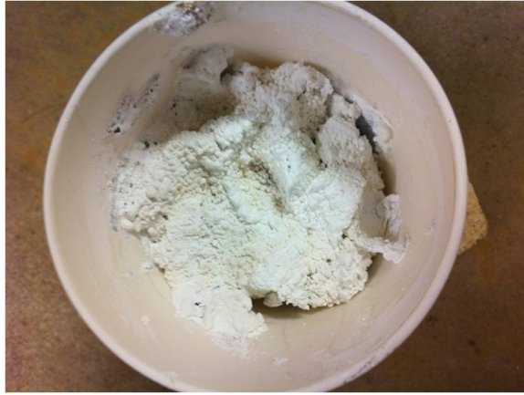
Figure 4.2. C_3S Crystals After Annealing at 1000C^\circ
