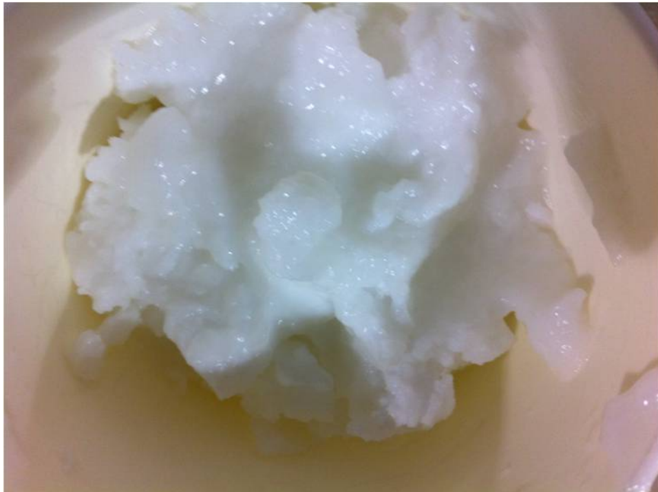
Figure 4.1. C_3S Paste Formed After Heating Solution to 100°C
