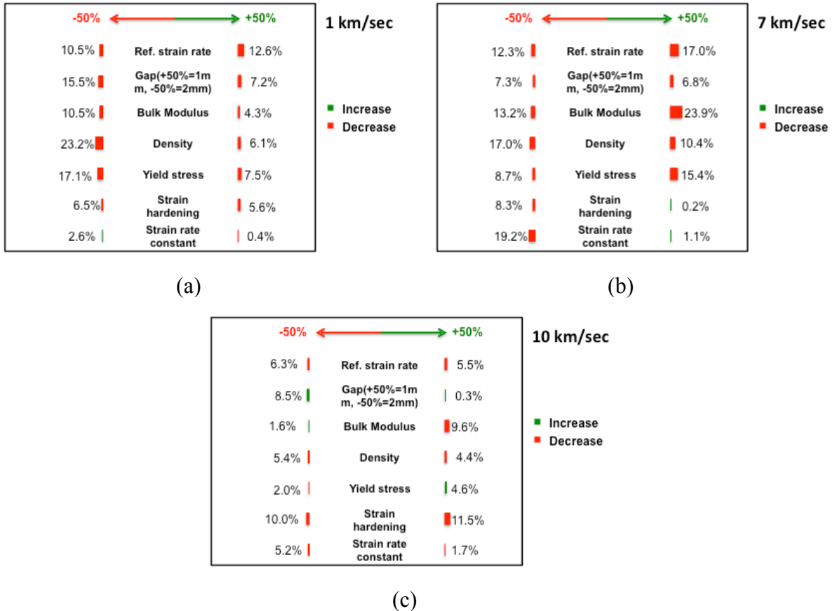
Figure 98: Crater diameter deviation from Steel substrate with reference coating after impact velocity of (a) 1km/sec (b) 7km/sec (c) 10km/sec
