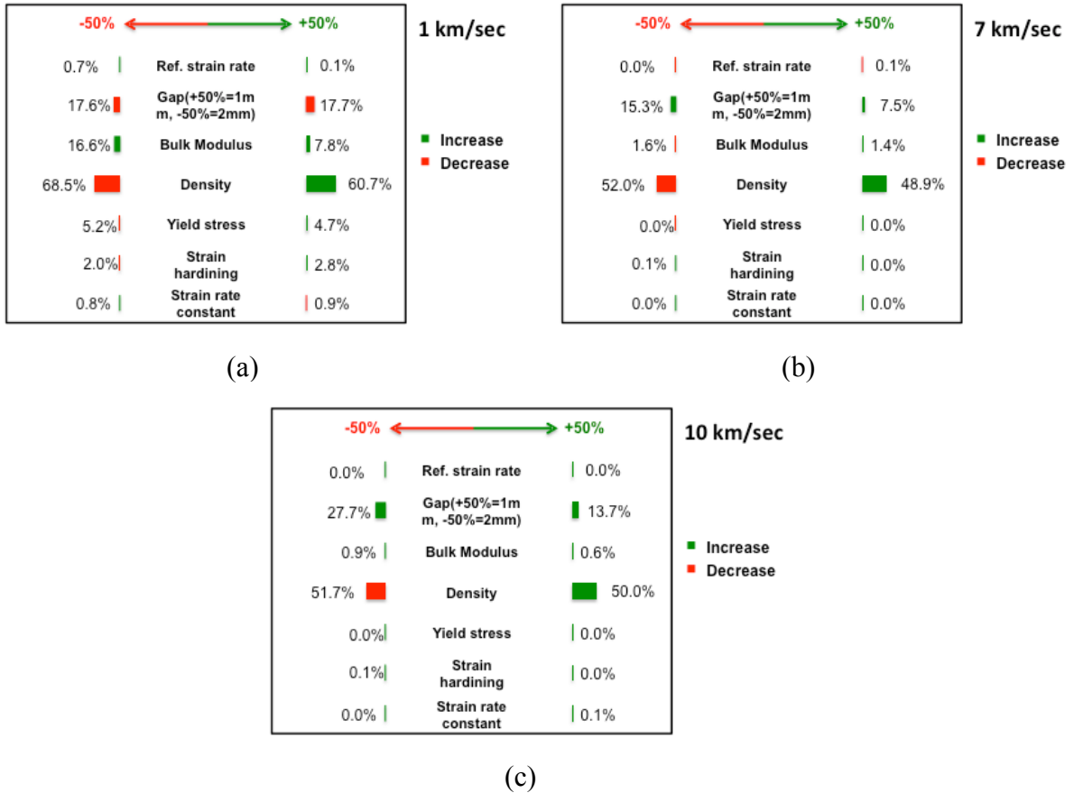
Figure 92: CNIP deviation from reference coating on Kevlar-Epoxy substrate after impact velocity of (a) 1km/sec (b) 7km/sec (c) 10km/sec
