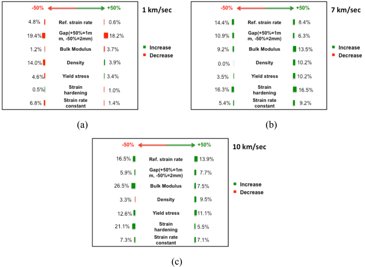
Figure 96: Crater diameter deviation from Aluminum substrate with reference coating after impact velocity of (a) 1km/sec (b) 7km/sec (c) 10km/sec
