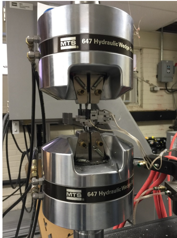
Figure 57: MTS and extensometer for stress-strain and Poisson's Ratio measurement
