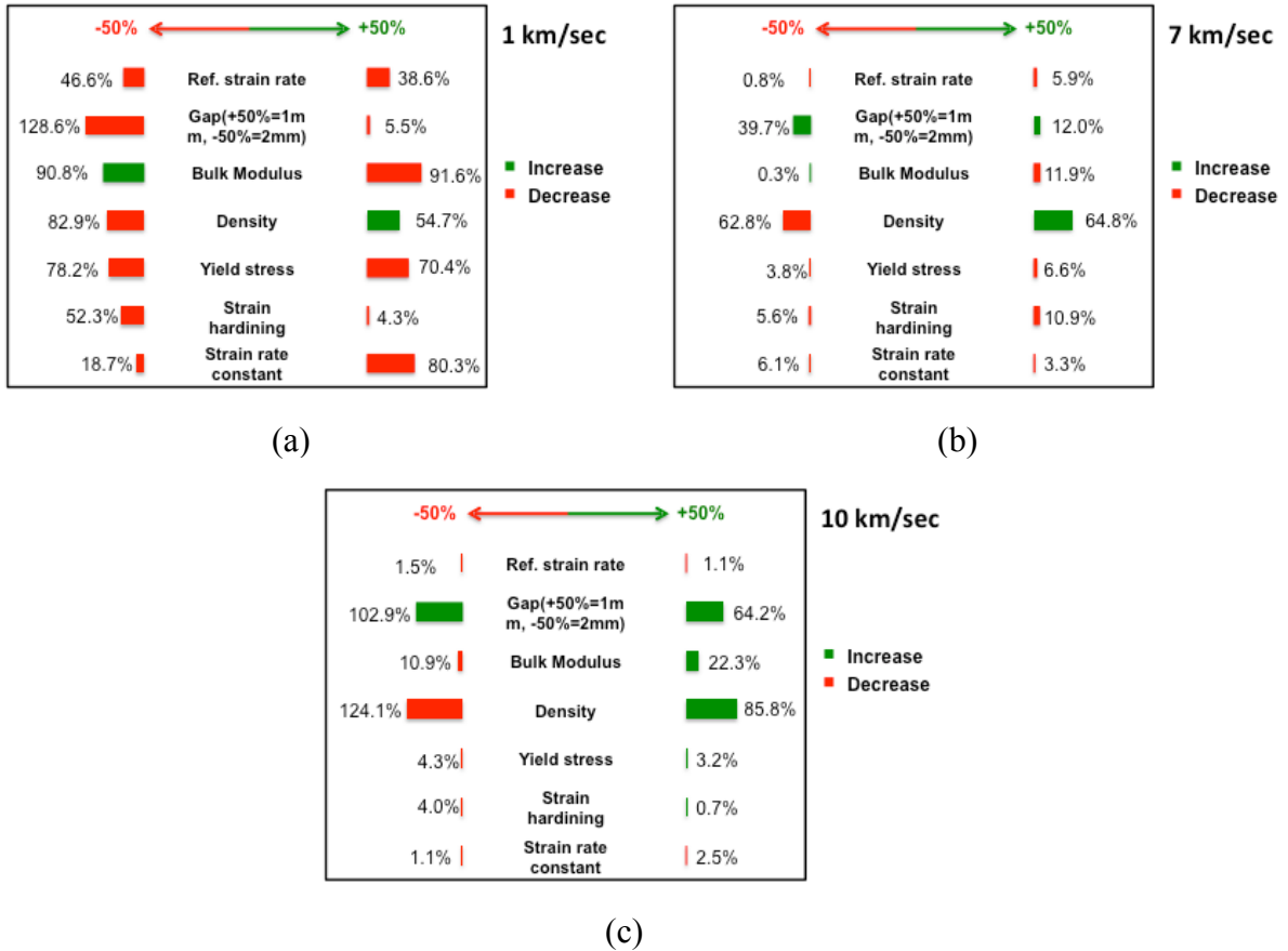
Figure 93: CNIP deviation from reference coating on Steel substrate after impact velocity of (a) 1km/sec (b) 7km/sec (c) 10km/sec
