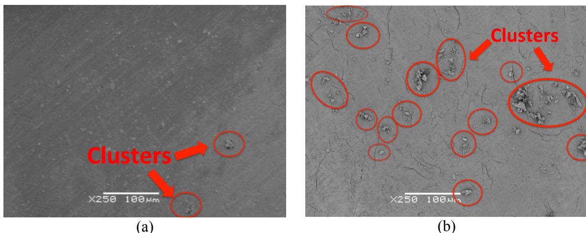
Figure 30: Typical SEM image (a) 3% xGnP (b) 3% OxGnP nano-composites
