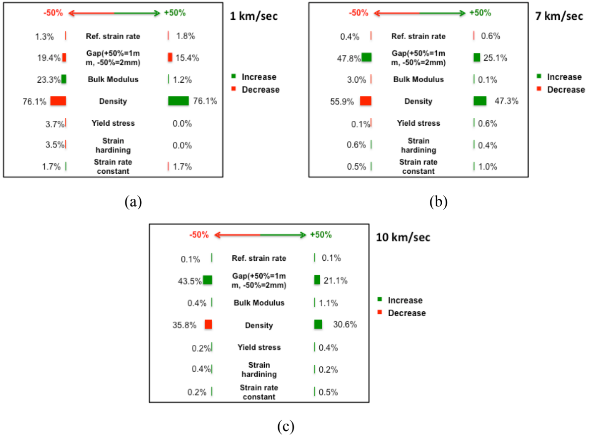
Figure 91: CNIP deviation from reference coating on Aluminum substrate after impact velocity of (a) 1km/sec (b) 7km/sec (c) 10km/sec
