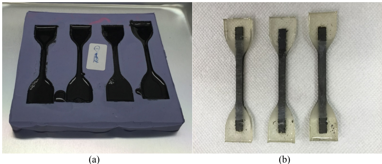
Figure 56: Dog bone shaped specimen (a) Roll-milled casted in silicon mold (b) Laminated tabbed with epoxy
