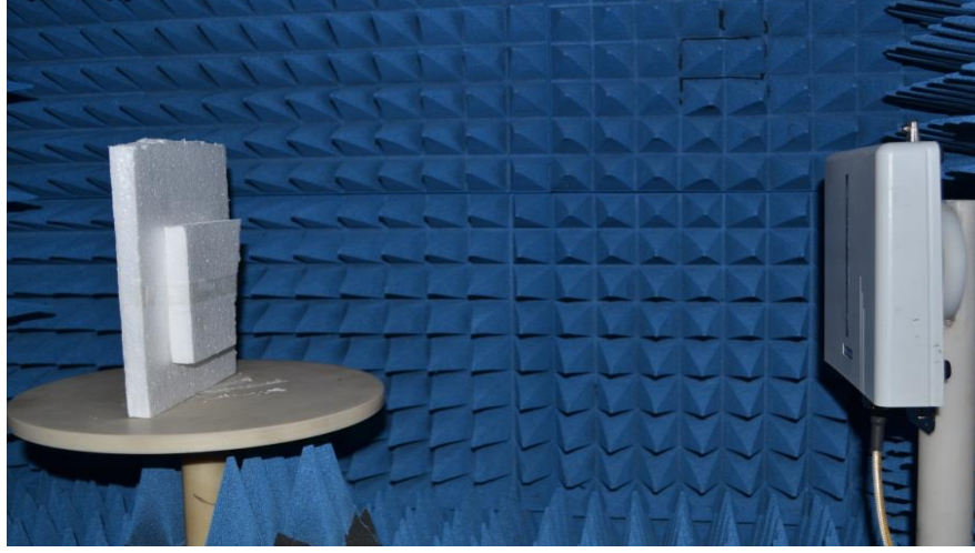
Fig. 4-13 Measurement Setup of measuring the HDPE-BST based RSA performance.
