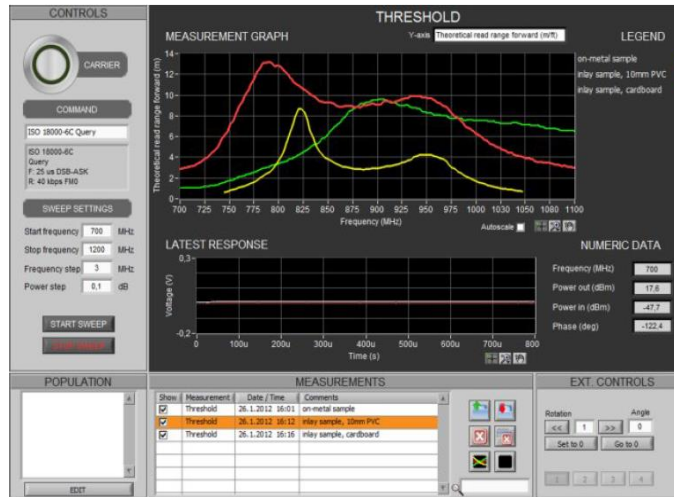
Fig. 3-6 The interface of measuring theoretical read range using the software.
