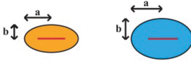
Figure 2.2. Cross section of the elliptical dielectric cylinders used for the cloaked antennas. The two elliptical cylinders shown here are representative of the final designs, where Antenna I has a smaller ellipse and Antenna II has the larger ellipse.
