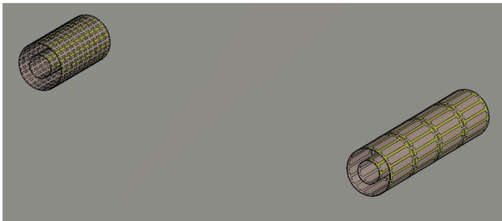
Figure 3.14. Geometry of the Cylindrical wideband antennas when placed at a distance d = 88 mm.
