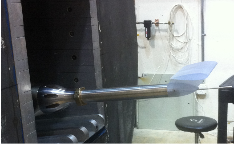
Figure 2.7. Airfoil Model Assembled on the Model Support System
