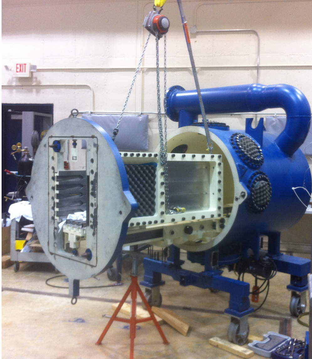
Figure 2.9. Installation of Windowed Walls into the Transonic Test Section
